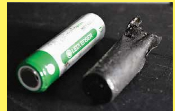
Cause of fire (lithium-ion batteries)
