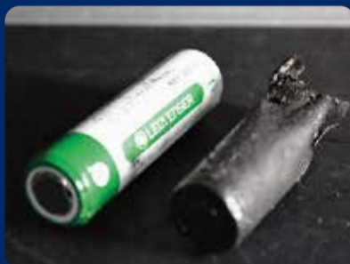
▲Cause of fire (lithium-ion battery)
