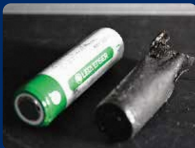
▲Cause of fire (lithium-ion battery)
