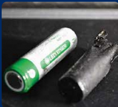
Cause of fire (lithium-ion battery)
